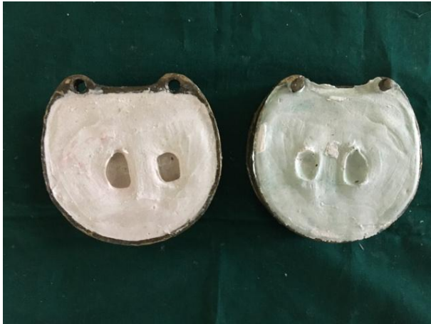
Figure 3: Resultant mold space after dewaxing
