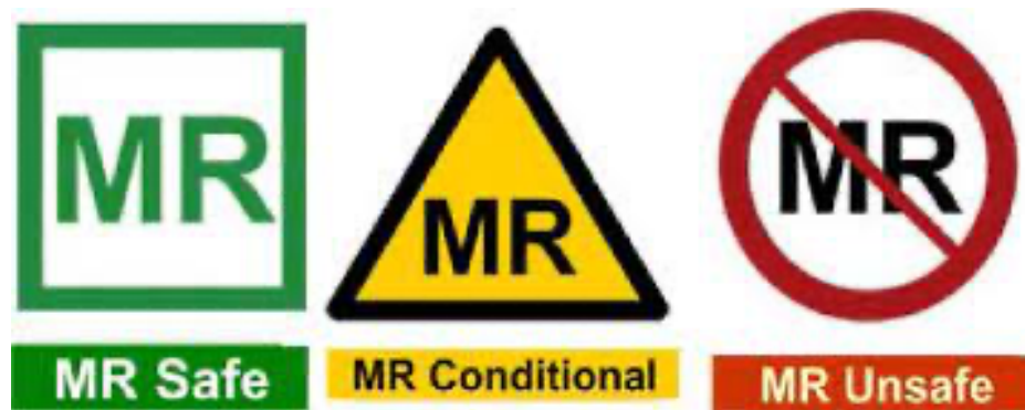
Figure 1: MR safety symbols of ASTM, classification in danger categories: green square: MR safe, yellow triangle: MR conditional, red circle: MR unsafe.
